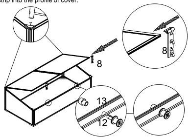
5 Cover Brackets & Bracket Seats Installation / Rear corner caps Installation
